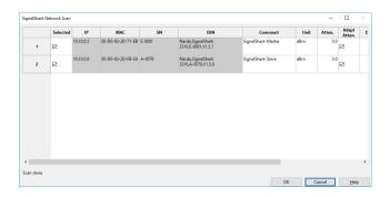
6. Click "OK" to save the information of all detected devices in the network in a json file "devicelist.json".
