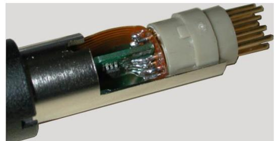
**Figure 3: A small memory chip in the NBM probe stores all the major probe data**
