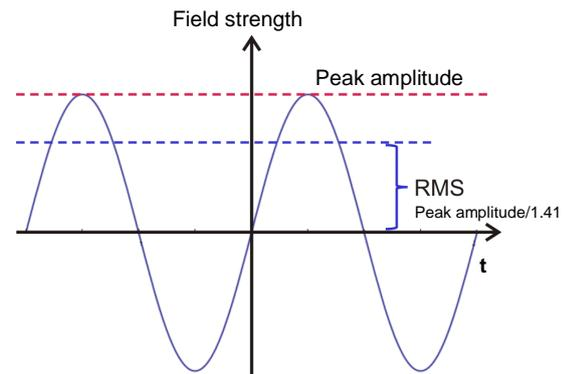
**Figure 1: RMS value of a sine wave field strength signal versus time**
