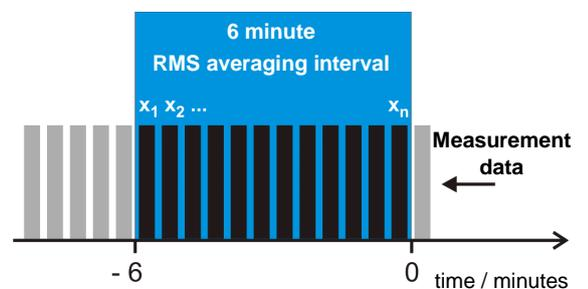
**Figure 4: Formation of the floating average field strength value using a continuous result memory**
