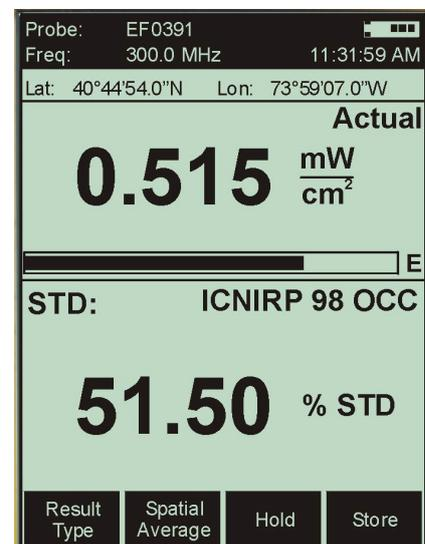
*Apply Standard: You can also display the field strength as a percentage of the limit value of a standard even when using flat probes. Simply select the standard on the NBM-550 (ICNIRP in the example shown) and set the frequency. The evaluation is useful if the main component of the field strength is due to a single source of known frequency. Available standards are listed on page 6.*
