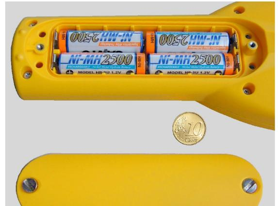
*Above:* The battery compartment is opened easily using a coin. Four replaceable NiMH rechargeable batteries (AA size) are used to power the device.
