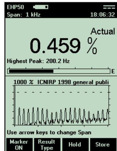
Standard mode displays the spectrum of the measured field, evaluated e.g. according to the ICNIRP guidelines. The dotted line represents the limit value (100%).
