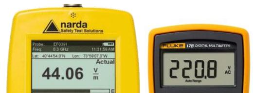
**Figure 2: Results are always displayed on the NRM as RMS values just like a multi-meter regardless of the result type setting**
