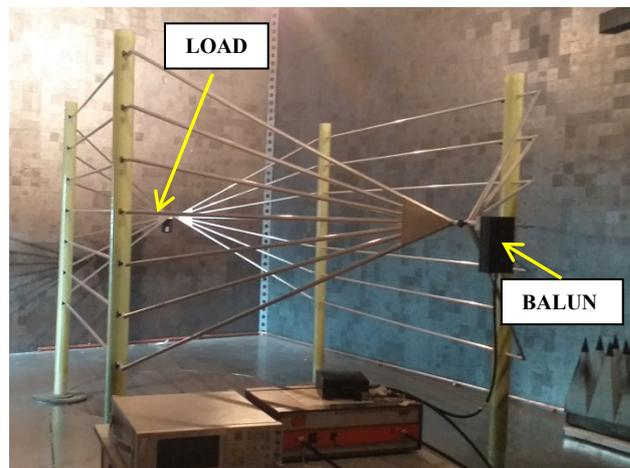
Fig. 3. A view of the Multi-Wire TEM transmission line in the setup employed during the experimental activities.
