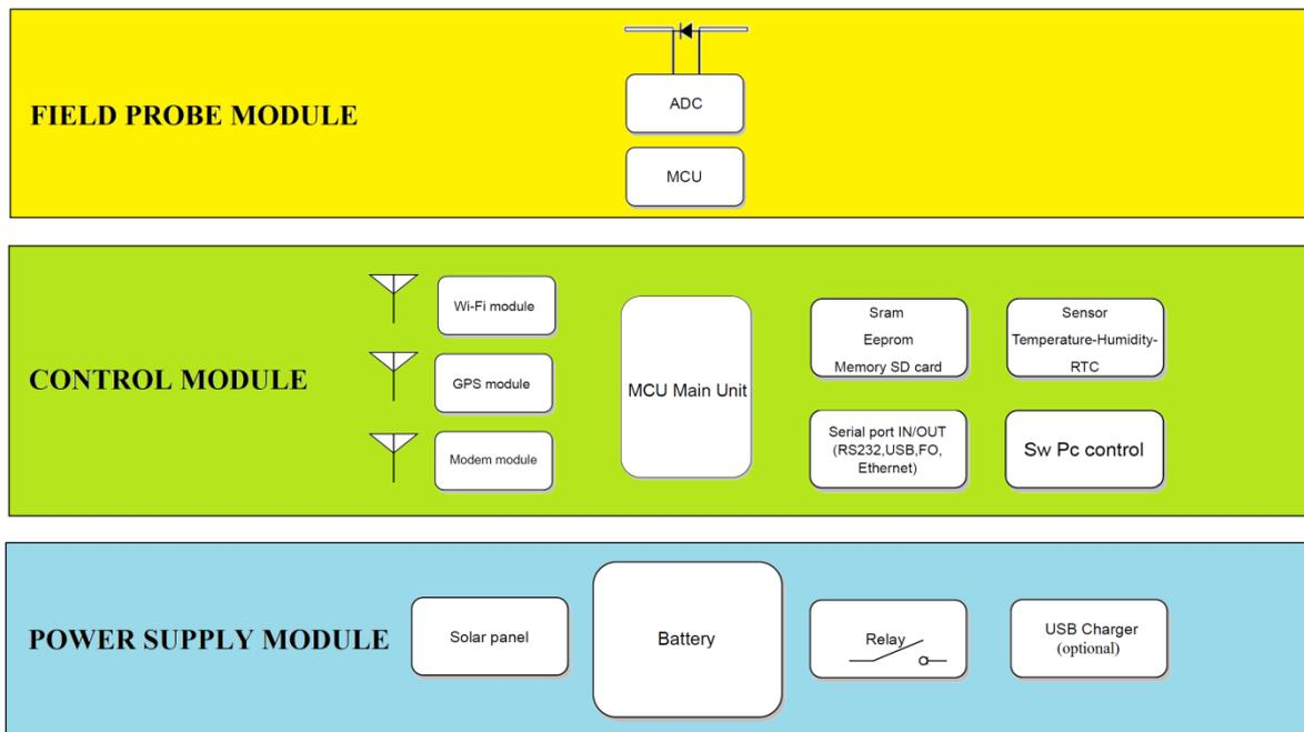
Fig. 2. Modules composing the NARDA AMB-8059 Area Monitor.
