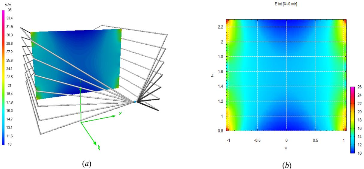
Fig. 4. Electric field simulated amplitudes in the central ( $x=0$ ) transversal section of the MWTEM transmission line ( $f = 20$  MHz,  $V_{rms} = 40,3$  V,  $Z = 58-j51$   $\Omega$ ): (a) field amplitudes and line geometry, (b) detailed plot of the field amplitudes.
