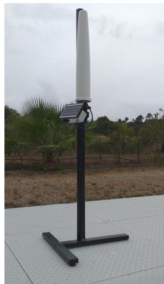
Fig. 1. An example of battery operated EMF Area Monitor (by courtesy of NARDA Safety Test Solutions S.r.l.).
