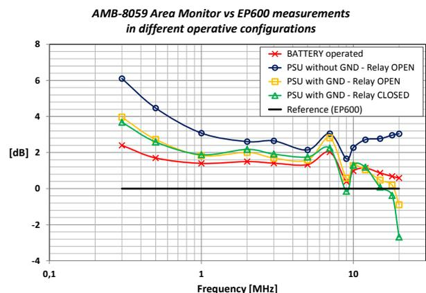
Fig. 6. Deviation of EMF Area Monitor measurement results from reference values in different simulated realistic conditions.
