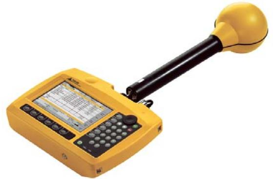
In *Scope* mode, the Selective Radiation Meter can display the time characteristic in real time of a signal captured using frequency selection. As with an oscilloscope, you can measure pulse widths and periodic times and set triggers. The settable time intervals range from 24 hours down to microseconds, with a resolution down into the nanosecond range.
