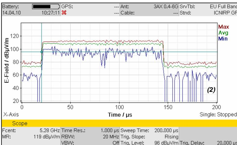
The blue "picket fence" representing the minimum values (1) may at first seem puzzling. This occurs because of the logarithmic scale of dBµV/m used for the Y-axis. If the minimum value falls below the detection threshold, it would be shown as zero on a linear scale, but on a logarithmic scale it is minus infinity!
