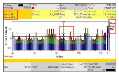
It's just as easy to use the bar graph display to see the actual occupancy of UMTS frequency channels. This means that users can see immediately which channels need to be demodulated and which do not. That saves measuring where there is nothing to measure.
