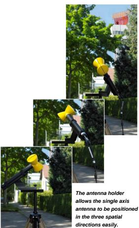
The antenna is simply fixed to the specially designed holder and turned from Position 1 to Position 2 and finally Position 3. While doing this, it is important that the position of the overall measurement setup (tripod, antenna, SRM, antenna holder, cable, person measuring) is not changed.
