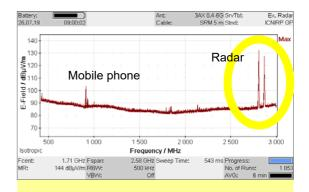
**Figure 1: Determining the radar frequency** In this case, the primary radar uses two channels at 2.808 GHz and 2.868 GHz. The channels transmit pulses alternately in order to achieve higher resolution without one channel saturating the receiver of the other channel in each case.
