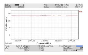
**Figure 8**: A zoom view of the main peak of the radar signal shows only a slight ripple if the resolution bandwidth is set correctly.
