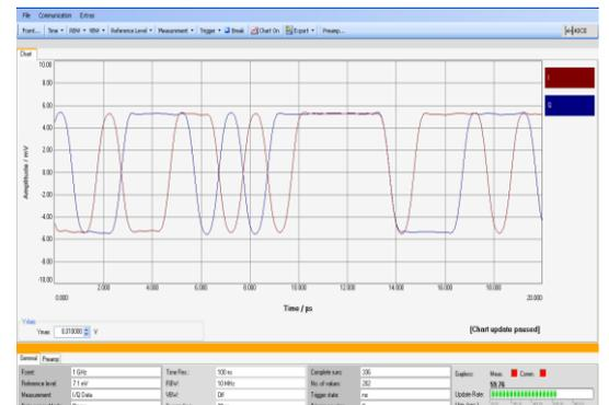
**IQ-Data-View for detailed analysis of digital modulated signals**
