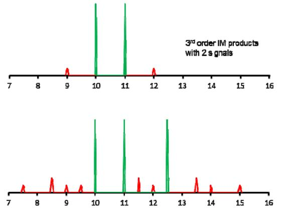
**Figure 5: 3<sup>rd</sup> order intermodulation products.**
