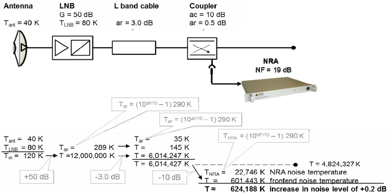
Figure 3: Determining the noise temperature
