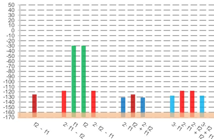
**Figure 9: SignalShark dynamic range for -30 dBm signals at 928 MHz and 929 MHz**
