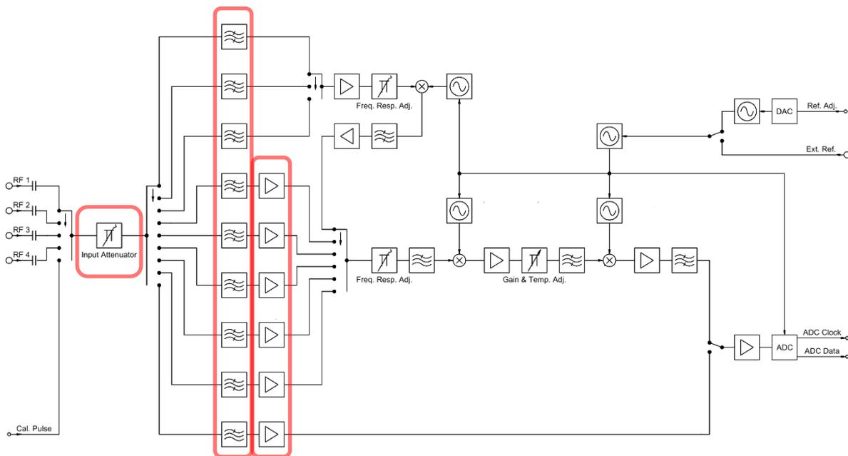
**Figure 6: High-performance RF front end of the SignalShark—high dynamic range due to suboctave filter bank (center), high quality IF amplifier (right) and attenuators that cover all frequency paths.**
