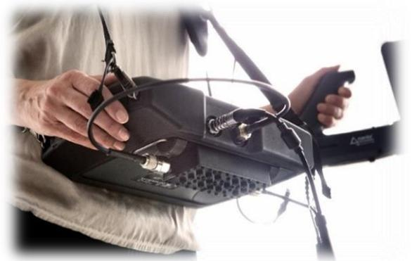
**Figure 10: External filter between antenna and receiver**
