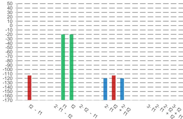
**Figure 8: SignalShark dynamic range for -20 dBm signals at 890 MHz and 2150 MHz**
