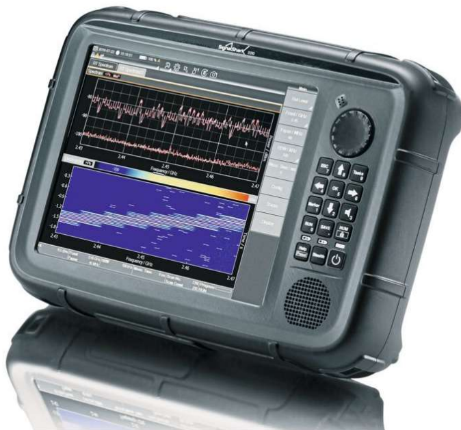
Figure 2: TE have been able to increase the frequency range for performance tests from 3 GHz to 8 GHz by using the new Narda SignalShark. At the same time, the overall handling of the antenna tests has been significantly streamlined because all the “intelligence” needed — apart from the electronic compass — is incorporated into a single device in the form of an inbuilt powerful computer.
