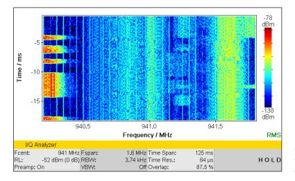
The downlink signal level drops strongly and the level of the in-house jammer rises as strongly inside the building. Figure 5 corresponds to the previous image but shows the entire 125 ms.
