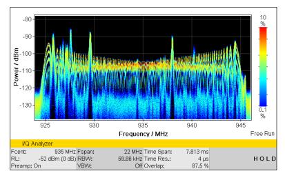
Figure 7: Gapless spectrogram. The weak signals can also be seen in the artificially generated blanking gaps in the jammer signal.
