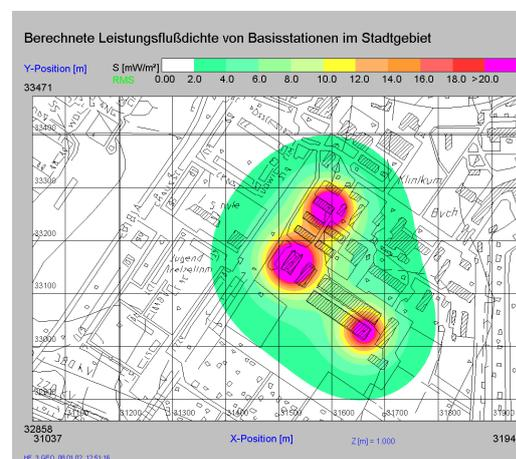
Fig. 3. Power flux density in an urban area
