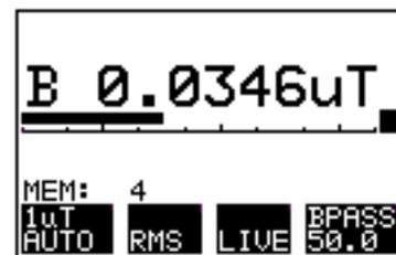
In broadband mode, the large, backlit display provides measurement and frequency results simultaneously.
