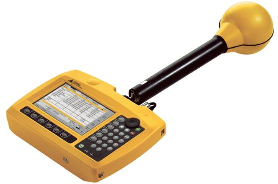
The Selective Radiation Meter SRM-3006 is equipped with *Safety Evaluation* mode, specifically designed for its special role in making environmental and safety measurements (Technical Note 01). Nevertheless, it can also be used generally just like a spectrum analyzer for making safety assessments as well. *Spectrum Analysis* mode provides various display and evaluation features for this purpose:
