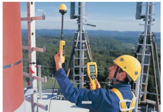
**Figure 7: Field strength measurement with a wideband probe.**
