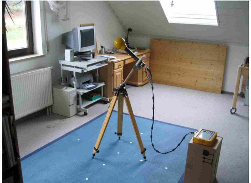
**Figure 8: Field strength measurements using the matrix method in an enclosed space [BOR 05-2].**
