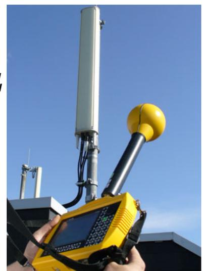
maximum values of the individual signals can then be taken from the *Max Hold* spectrum for further evaluation. However, the antenna must be moved slowly in relation to the measurement speed of the spectrum analyzer.
