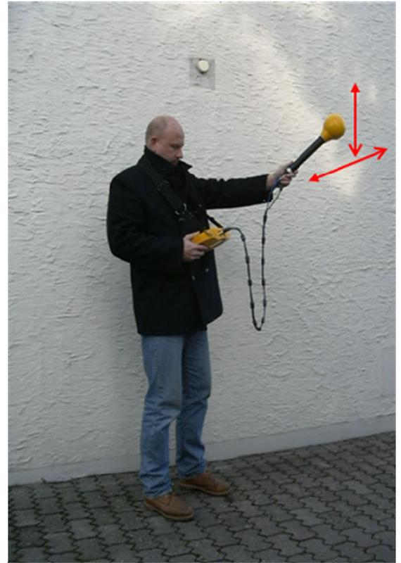
**Figure 4: Searching for local field strength maxima using the pendulum method.**
