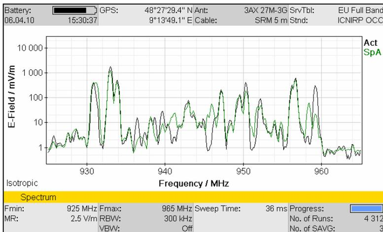
**Figure 2: Example of an analysis of the GSM-900 spectrum using Spatial Averaging. The values at specific frequencies can be read off numerically using the marker. The SRM-3006 can also automatically list the highest values with their corresponding frequencies in the Peak Table.**
