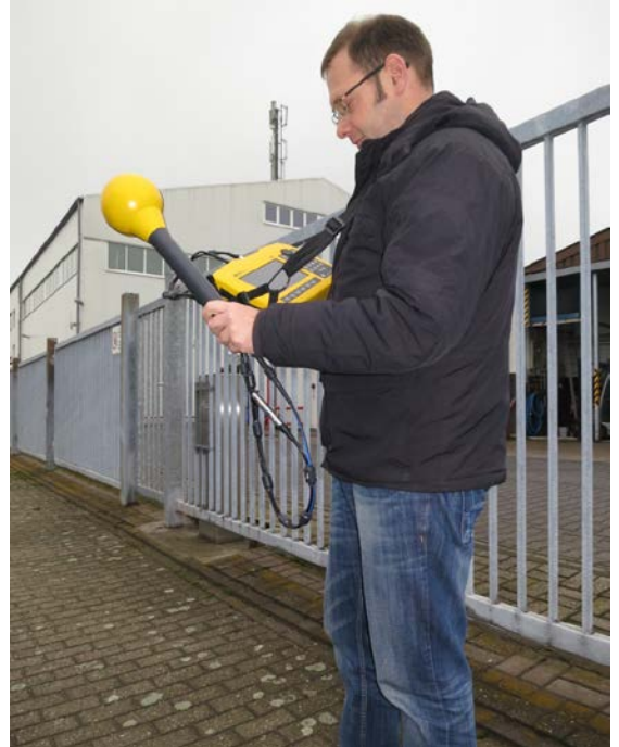
Figure 2: LTE measurement with the SRM-3006 and an isotropic antenna.
