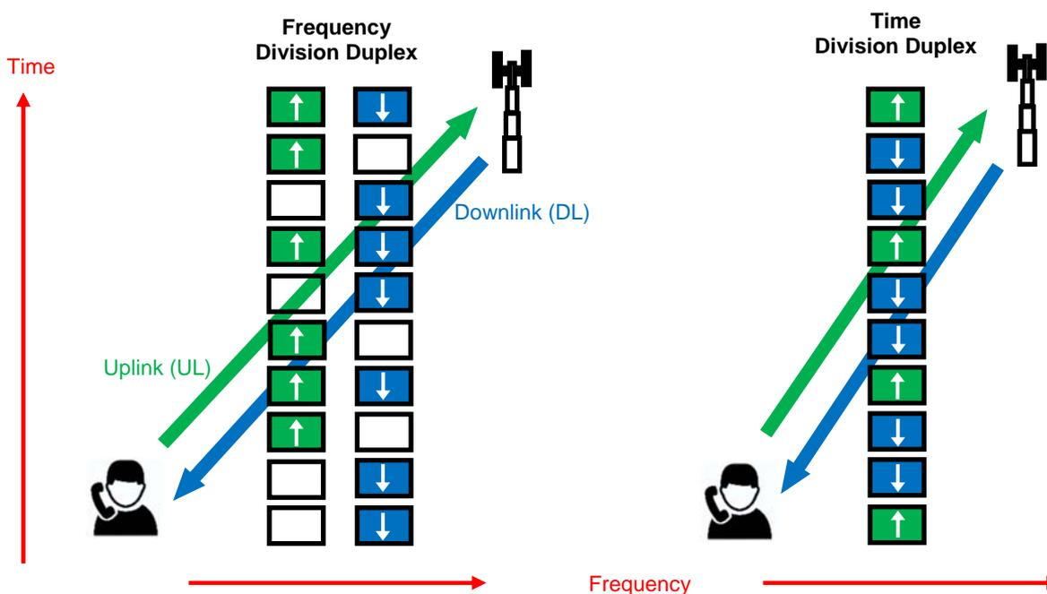
**Figure 2: The difference between FDD (left) and TDD (right)**
