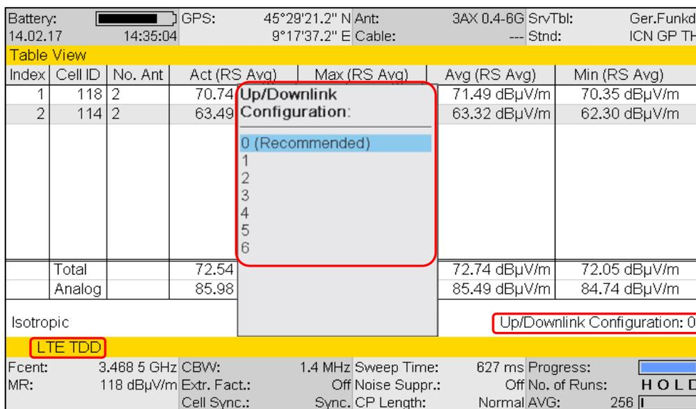
**Figure 4: LTE TDD option in the SRM 3006 with uplink / downlink configuration selection**
