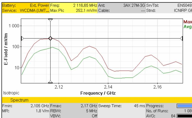
**Figure 2: Spectrum Analysis of the UMTS frequency range using a low resolution (RBW = 5 MHz). The channel power can now be read off directly using the Peak Marker. A special algorithm ensures that the peak marker is placed exactly on the channel maximum.**
