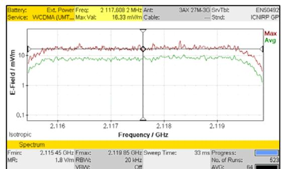
**Figure 3: To find the center frequency, zoom in to one UMTS frequency channel from the spectrum shown in figure 1. Adjustment of the marker is then much easier. Nevertheless, some manual adjustment to the actual center frequency may be necessary in UMTS mode.**
