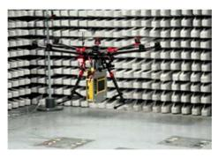
Figure 3: Drone in flight above the test turntable with active measuring device control during immunity testing (without isotropic antenna)
