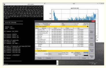
Figure 1: Remote control of the SRM 3006 from the ground station
