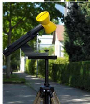
*The antenna holder allows the single axis antenna to be positioned in the three spatial directions easily.*
