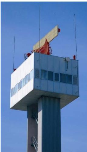
**A typical antenna array: a parabolic antenna for the primary radar beneath a linear dipole array for the secondary radar. Both antennas rotate together.**
