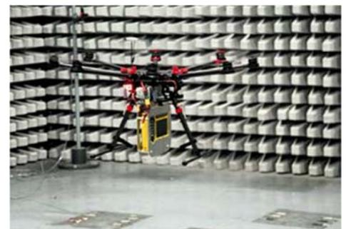
Figure 3: Drone in flight above the test turntable with active measuring device control during immunity testing (without isotropic antenna)
