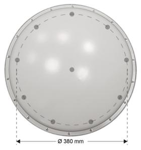
Figure 6. Large aperture uniform circular antenna array with 9 elements and an additional reference element in the center as used in the ADFAs for frequencies from 200 MHz to 2.7 GHz
