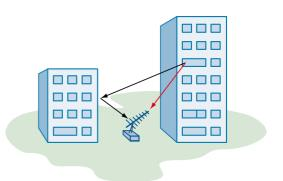
Figure 5. Multipath propagation from a transmitter in the taller building to the receiving antenna on the floor
