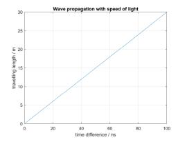
Figure 15. Travelling length versus time difference for speed of light
