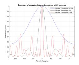
Figure 7. Beamform of a uniform circular antenna array with 9 elements for diameter to wavelength ratios of 0.24, 1, and 3.6
