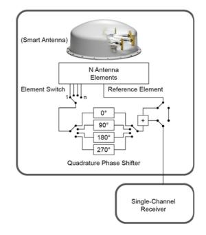
Figure 11. Single channel correlative interferometer
