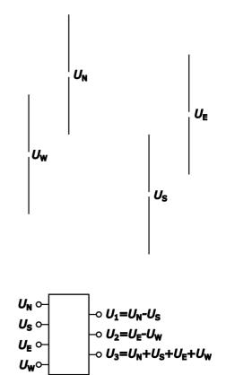
Figure 10. Adcock antenna array
