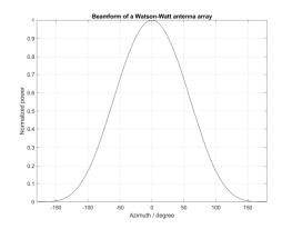
Figure 9. Beamform of a Watson-Watt antenna array
