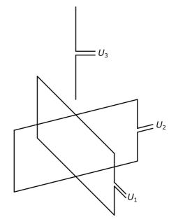
Figure 8. Watson-Watt antenna array
