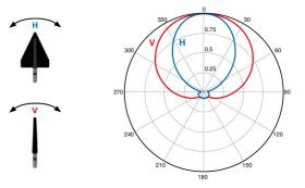
Figure 2. Directional pattern of a logarithmic periodic antenna
