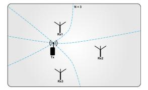
Figure 14. Three receivers localizing a transmitter using TDoA hyperbolas
