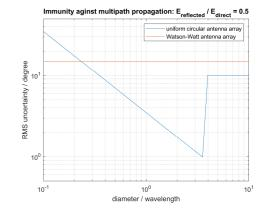
Figure 12. Immunity against multipath propagation for a uniform circular antenna array with nine elements and for a Watson-Watt antenna array
