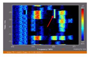
High Resolution Spectrogram Zoom of GSM downlink traffic showing a 4 ms segment from a total time span of 62.5 ms. Time resolution is 16  $\mu$ s. The illegal transmitter can be seen immediately, as its duration does not correspond to the normal GSM timeslot length of 546  $\mu$ s.
