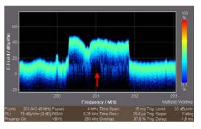
The same signal in a Persistence Spectrum obtained from the same I/Q data set. The interference is visible here, too: At around 201 MHz, the signal level does not drop to around the noise level as expected.
