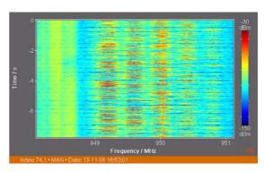
A "normal" GSM downlink traffic spectrum, obtained in Spectrum mode with 20 ms resolution.
