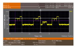
A GSM downlink signal shown in Magnitude display mode, triggered on the rising edge. Time resolution is 2  $\mu$ s. The 546  $\mu$ s timeslots can be clearly seen and the frame duration can be measured using markers A and B:  $\Delta t = 4.616$  ms.
