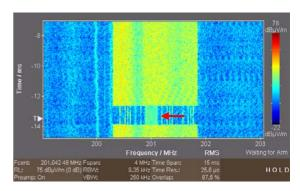
High Resolution Spectrogram Zoom of a DAB channel, triggered on the null character. The interferer can be clearly seen in the gap.
