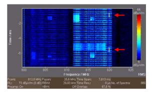
High Resolution Spectrogram Full of two LTE channels. Resolution 8 µs. The frame structure is clearly seen – practically a textbook image – with its resource grid and synchronization signals.
