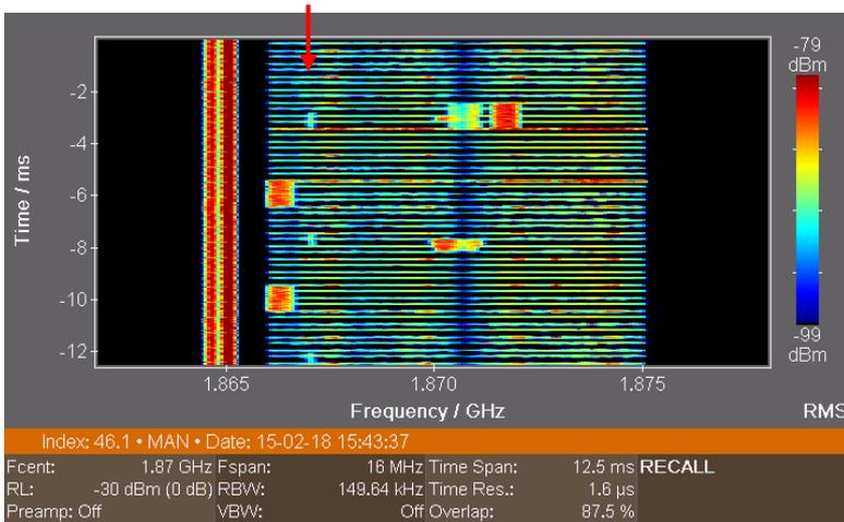
**Figure 4: High-Resolution Spectrogram Full. Bandwidth (Fspan) 16 MHz, frequency resolution (RBW) approx. 150 kHz, time resolution 1.6  $\mu$ s. The instrument only compresses the data for display to match the screen resolution, but the original data is retained.**
