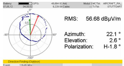
**Figure 7. Using a Horizontal Scan to find the bearing of T008 in a northerly direction from the location of the IDA-3106 south of the runway as determined by GPS.**
