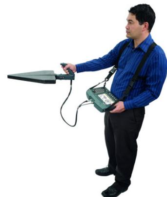
**Figure 9. Performing a Horizontal Scan with IDA-3106 to find the bearing of a transmitter.**
