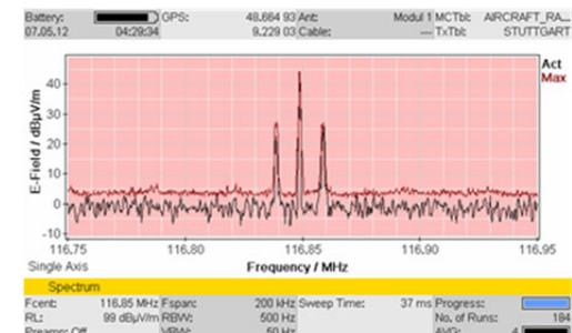
**Figure 4. Suspect transmitter T008 at 116.850 MHz displayed at high frequency resolution shows the typical sidebands of amplitude modulation**
