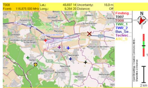
**Figure 10. RF transmitter map with localization of all transmitters and signals of interest**
