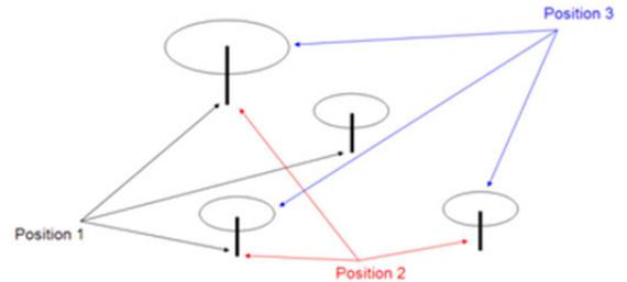
**Figure 6. Diagram of the principle of taking cross-bearings on several transmitters, all operating at different frequencies**
