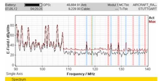
**Figure 3. Highlighted entries in the Transmitter Table ready for further detailed investigation**
