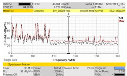
**Figure 2. Actual FM and aircraft radio band usage at Stuttgart Airport, with an initially unidentified transmitter marked at 116.875 MHz**
