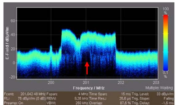
**The same signal in a Persistence Spectrum obtained from the same I/Q data set. The interference is visible here, too: At around 201 MHz, the signal level does not drop to around the noise level as expected.**
