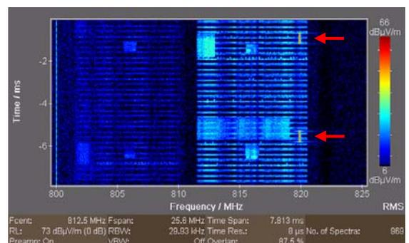
**High Resolution Spectrogram Full of two LTE channels. Resolution 8  $\mu$ s. The frame structure is clearly seen – practically a textbook image – with its resource grid and synchronization signals. The repeating interference, naturally, does not fit.**
