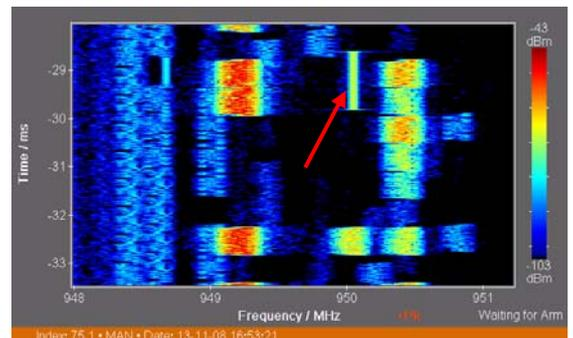
**High Resolution Spectrogram Zoom of GSM downlink traffic showing a 4 ms segment from a total time span of 62.5 ms. Time resolution is 16  $\mu$ s. The illegal transmitter can be seen immediately, as its duration does not correspond to the normal GSM timeslot length of 546  $\mu$ s.**
