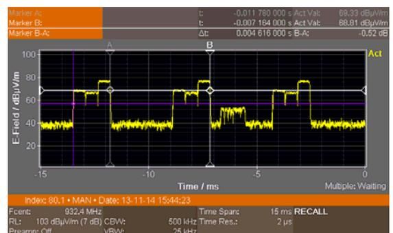
**A GSM downlink signal shown in Magnitude display mode, triggered on the rising edge. Time resolution is 2 μs. The 546 μs timeslots can be clearly seen and the frame duration can be measured using markers A and B: Δt = 4.616 ms.**
