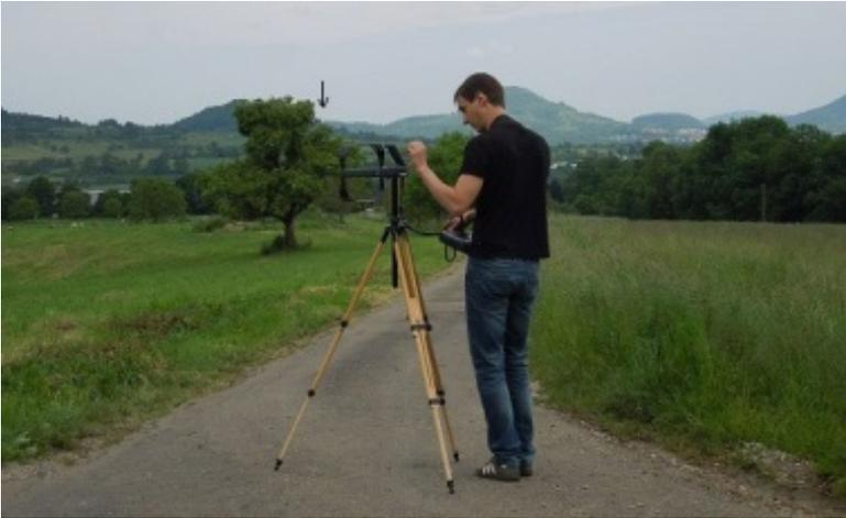
**Figure 3: Recording a horizontal scan in an open space. The conditions for taking bearings on the FM transmitter are ideal. Vertical polarization was selected here as an experiment. Normally, DAB transmitters are vertically polarized and analog FM transmitters horizontally polarized.**
