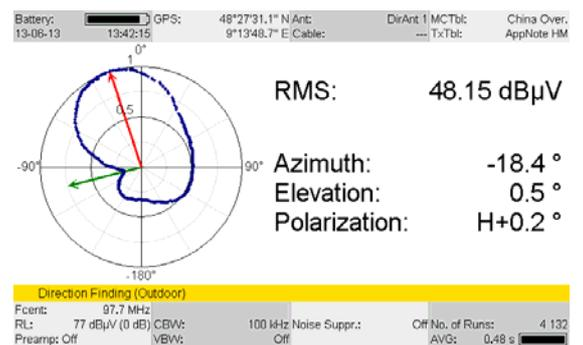
**Figure 5 – Bearing 2: Reflection effects. The red arrow indicates the calculated direction. The green arrow indicates the direction in which the antenna is currently pointing. From this direction, the reflections almost obliterate the signal.**
