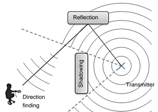
**Figure 4: Shadowing and reflection during direction finding.**
