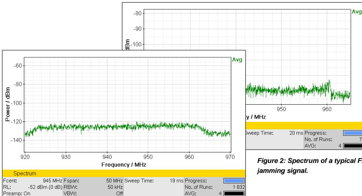
**Figure 1: Downlink suppression by increasing the noise floor.**
