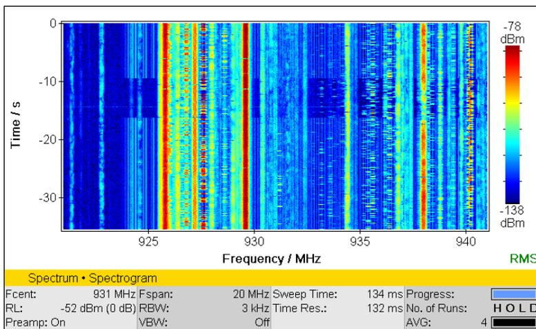
**Figure 3 Jammer signal shown as a conventional spectrogram.**
