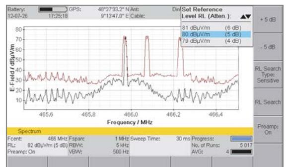
**Figure 5: Using the  $\pm 5$  dB offset makes it easy to distinguish between the actual signal and an intermodulation product. The reference level also determines the input attenuation.**
