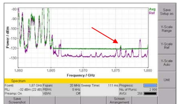
**Figure 4: The ideal balance between noise and intermodulation is achieved with 22 dB input attenuation (green). This allows you to distinguish intermodulation from the true measurement signal (red arrow). The spectrum from Figure 2 is again used as reference (violet).**
