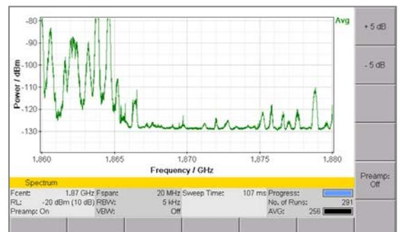
Figure 2: There appear to be several interferers present above the 1800 MHz mobile phone band. They are actually intermodulation products caused by non-linearities due to the input attenuation being too low.
