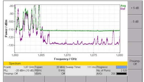
**Figure 3: High input attenuation causes increased noise (green). The spectrum shown in Figure 2 was saved as a reference (violet).**
