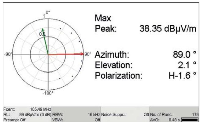
Bearing diagram from seven separate hand-picked measurements
