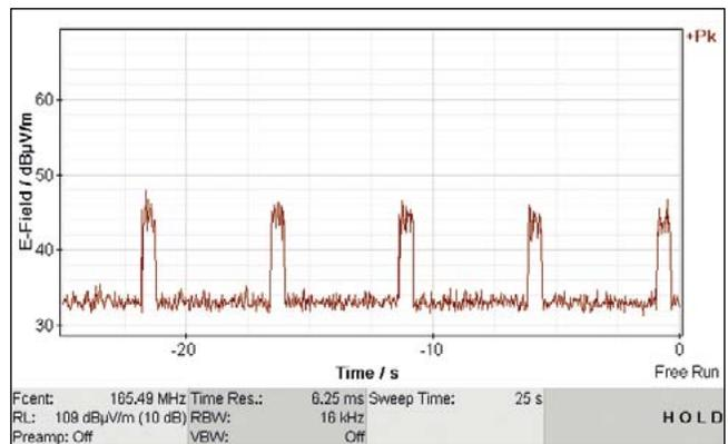
Scope Mode shows the amplitude versus time of the interfering signal
