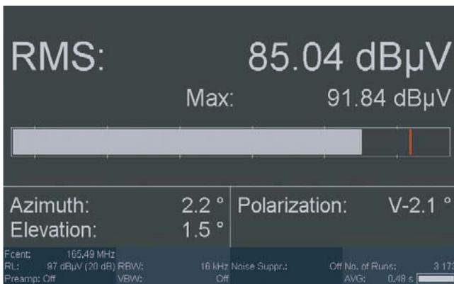
The bar graph and the Tone Search feature help narrow down the last few meters. The Night setting allows dazzle free viewing of the display even in the dark.
