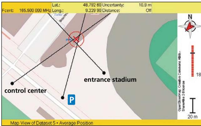
Triangulation from three bearings: 1. Bearing from the control center.
