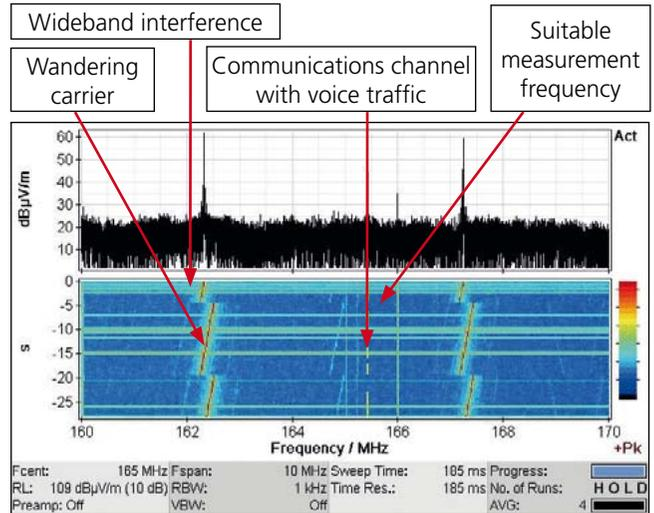
Combined display of spectrum and spectrogram
