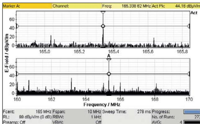
An initial overview from the control center shows the allocation and several interferers (below). The Magnifier takes a closer look at the area around the Marker (above).
