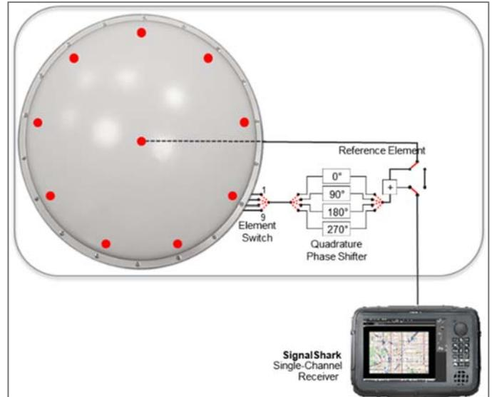
Fig. 2. Basic configuration of the single channel ADFA direction finding antenna.
