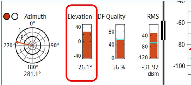
Fig. 1. Display of elevation during a measurement with the SignalShark and ADFA.
