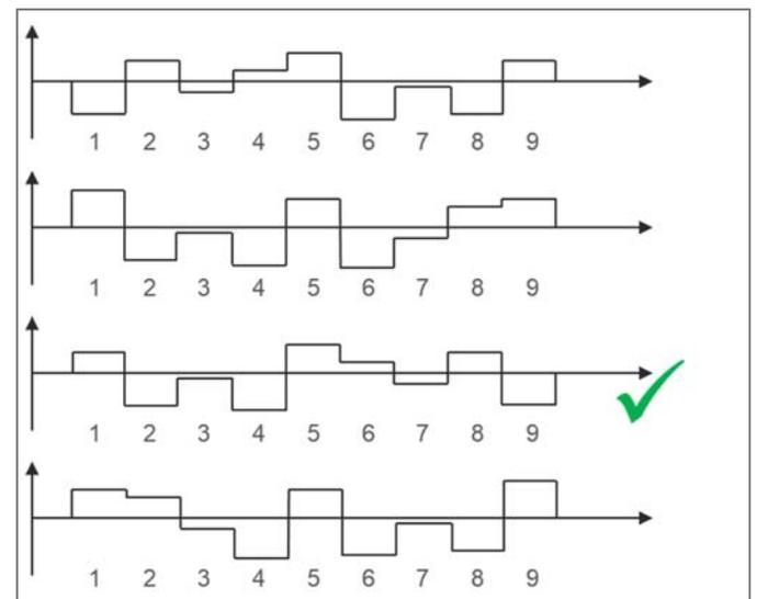
Fig. 4. Catalog of possible phase angle patterns stored in the SignalShark.
