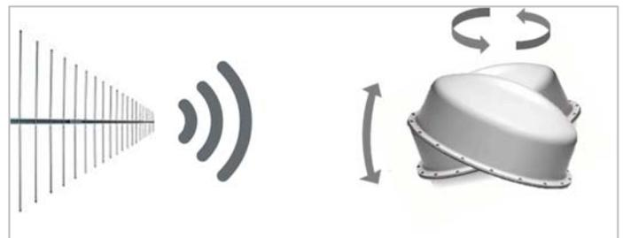
Fig. 7. Narda antennas are both rotated and tilted during the determination of the phase catalog.
