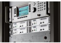
The SignalShark can, of course, be integrated into a large monitoring system as a rack mounted version or outdoor unit, for example. It delivers the essential standardized IQ data in Vita49 format.
