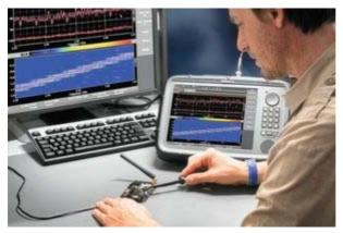
The SignalShark portable analyzer detects, analyzes, classifies and localizes RF signals between 8 kHz and 8 GHz. (Image: Narda STS)
