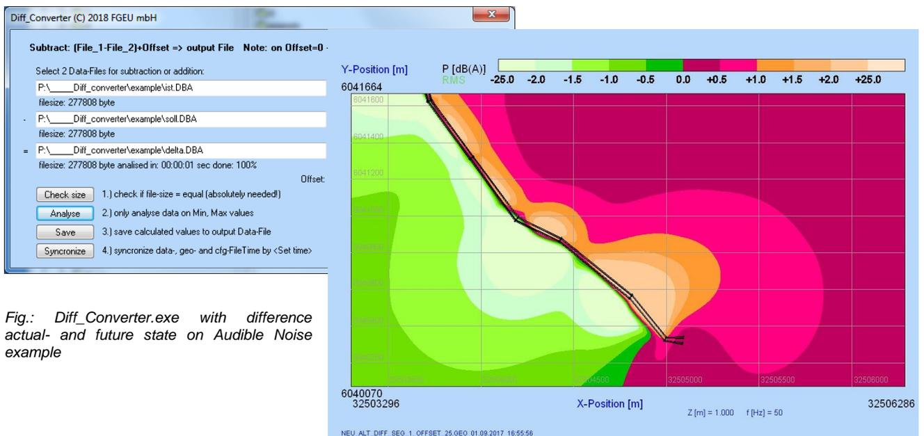
Fig.: Diff\_Converter.exe with difference actual- and future state on Audible Noise example
