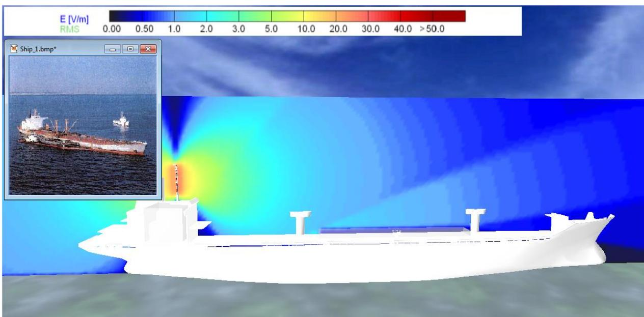
Fig.: new example of a container ship with antenna system
