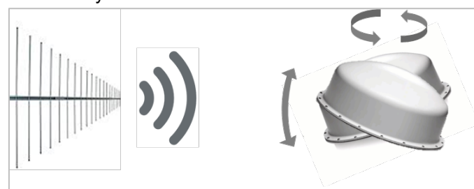
Fig. 9. Narda antennas are both rotated and tilted during the determination of the phase catalog.
