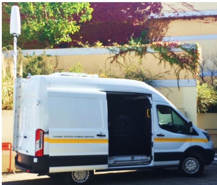
Figure 8: Diakar EMF safety evaluation vehicle equipped with Narda EMF antenna
