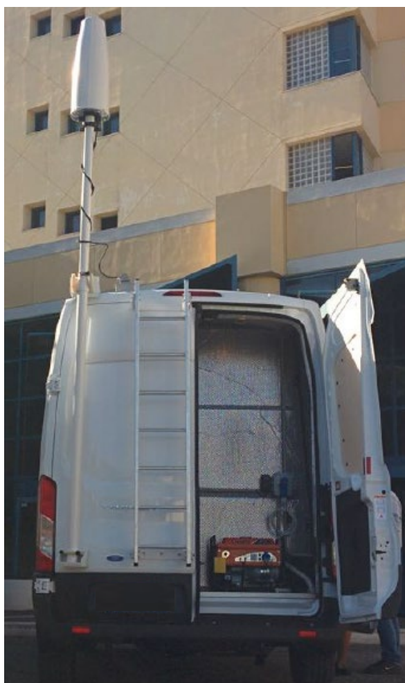
Figure 9: EMF safety vehicle by Diakar with detachable EMF antenna and safe storage compartment
