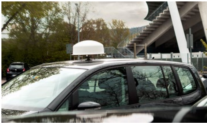
Figure 3: ADFA with magnetic mount on a rental car, operated from a SignalShark Handheld Unit to give non-permanent integration
