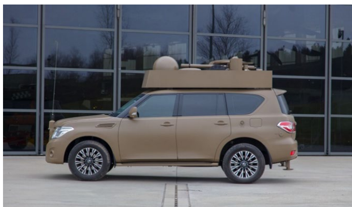
Figure 5: Teradium SF5 based on a Nissan Patrol SUV
