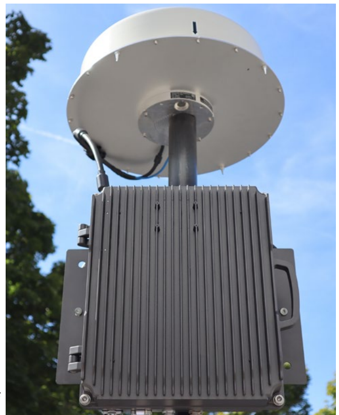
Figure 4: ADFA and SignalShark Outdoor Unit mounted close together on a mast and powered from PoE
