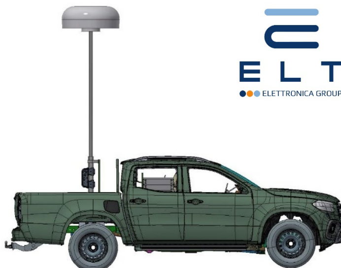
Figure 11: MUROS based on an SUV, with elevated mast
