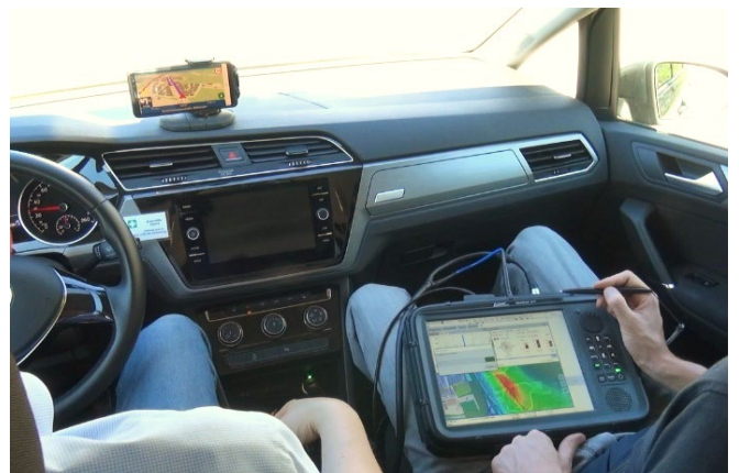
Figure 3: ADFA with magnetic mount on a rental car, operated from a SignalShark Handheld Unit to give non-permanent integration
