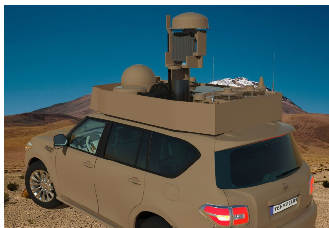
Figure 6: CAD drawing of Teradium SF5, showing SignalShark on elevated mast in the field without sunshield
