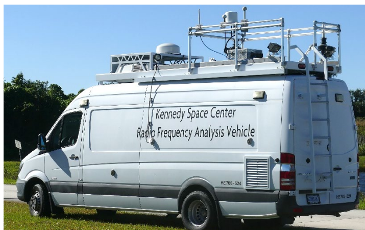
Figure 7: Radio monitoring vehicle at Kennedy Space Center equipped with SignalShark and ADFA 2
