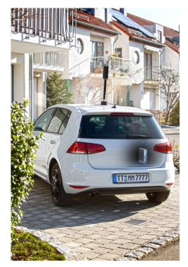
The fixed network installation can be expanded if required by means of mobile TDOA or AOA stations. This is illustrated here by fitting an omnidirectional antenna onto the roof of an automobile by means of a magnetic base. The SignalShark Remote Unit is fitted in the trunk. This setup is also excellent for independent spectrum monitoring or coverage measurements.
