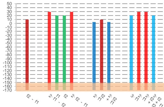
Bild 9: THI, Signal 19,77 dBm, Att 0 dB, RL -10 dBm
