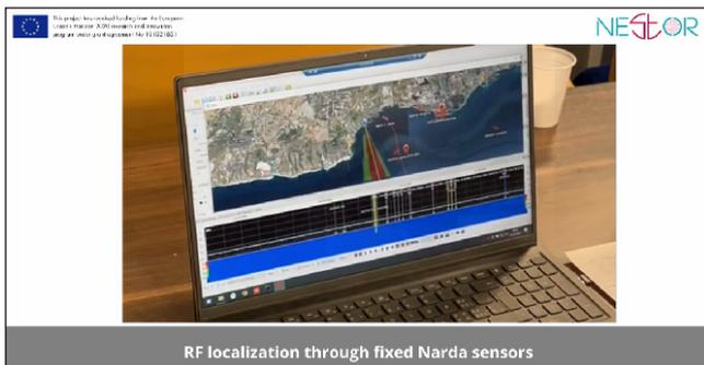
The test clearly showed that the additional use of radio frequency direction finding helped to locate shipwrecked persons significantly faster and more efficient compared to searching with traditional means such as cameras or from helicopters.
