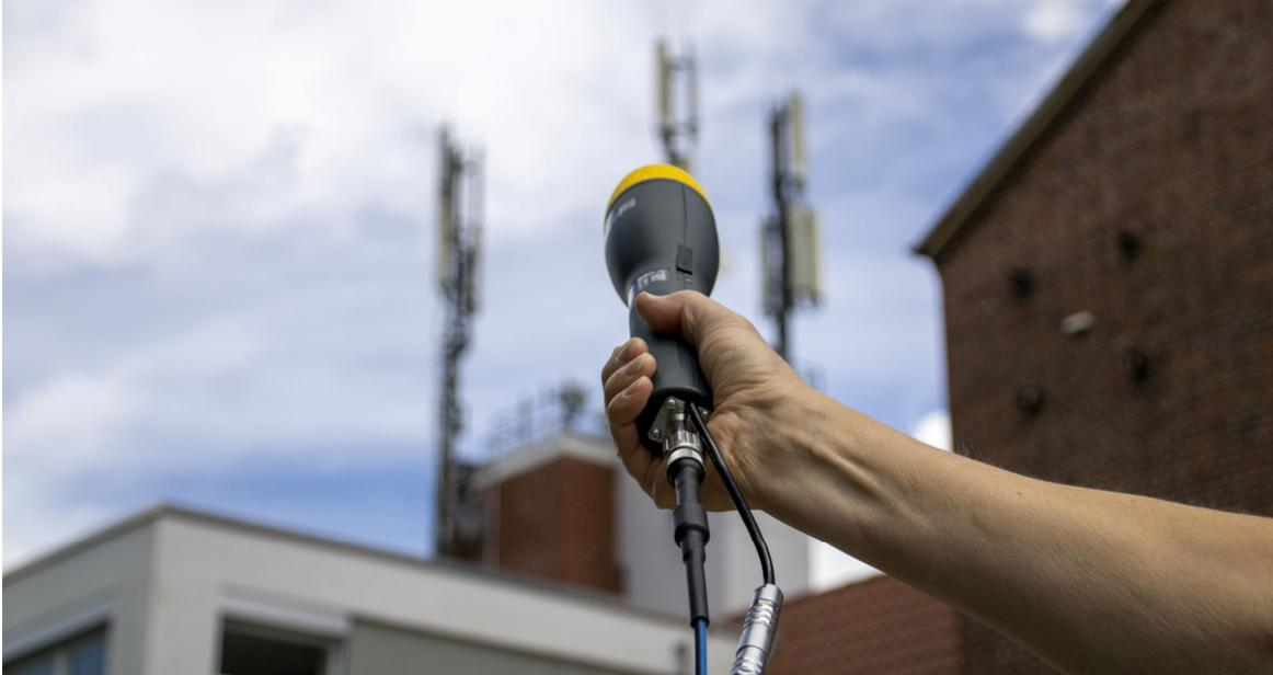
2. Omnidirectional antenna: Pointing it vertically into the sky
