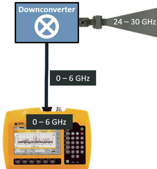
It's down converting mm-Waves into mid-frequency range so that the signal can be more easily transported and processed.
