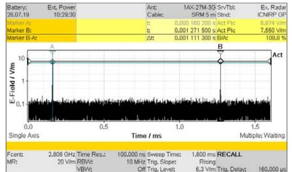
**Figure 4: Scope Mode, determining the pulse repetition frequency PRF**
