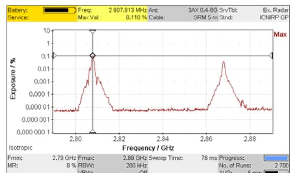
**Figure 2: Zoom for more precise determination of the radar frequencies**
