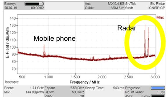
**Figure 1: Determining the radar frequency**
