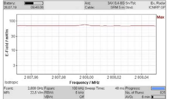
**Figure 8:** A zoom view of the main peak of the radar signal shows only a slight ripple if the resolution bandwidth is set correctly.
