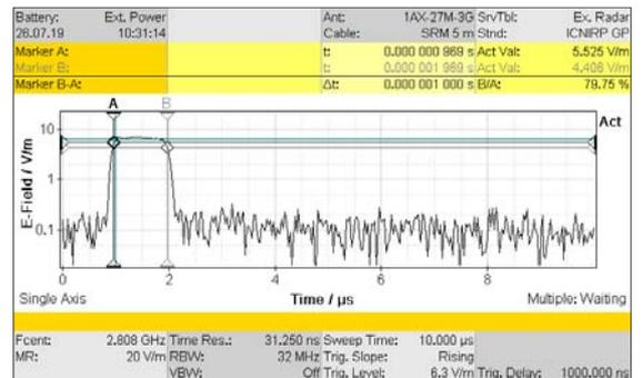
**Figure 5: Scope Mode, determining the pulse length**
