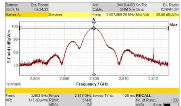
**Figure 7: Real spectrum of a radar signal.**
