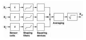
Block circuit diagram of ELT-400 with isotropic probe: The sensor coils detect the field in all three spatial directions simultaneously. Filters then shape the measured values according to frequency to correspond to the ICNIRP limit value curves. Squaring devices produce the power sum, which is then averaged and the square root taken to give the weighted flux density.
