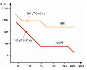
The ELT-400 from Narda Safety Test Solutions evaluates the magnetic flux density according to ICNIRP General Public. The IEEE limit value curves (yellow) are generally above the ICNIRP values (red) in the low frequency range. Devices that comply with ICNIRP will therefore also conform to the IEEE standard.
