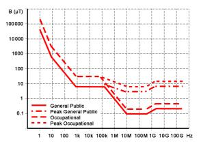
ICNIRP limit value curves for magnetic flux density
