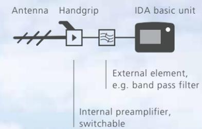
The overmodulation resistance of the preamplifier means that it is possible to insert a filter between it and the basic unit. The IDA 2 can store all the relevant transfer factors in the signal chain, from the antenna conversion factor to the preamplifier, filter, external attenuators and RF cable, and takes them into account together with the transfer function of its input stage when displaying the results.
