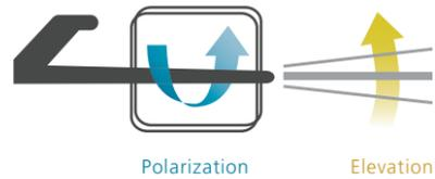
Position sensors in the handgrip determine the polarization and the elevation as well as the azimuth of the antenna.
