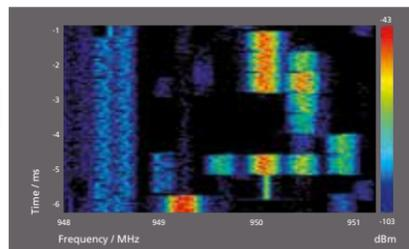
The spectrogram allows an overview of the entire signal sequence that is captured. The color values indicate the signal levels. Up to 8000 spectrums are combined into one view in this way. Even the briefest of impulses in the microsecond range are reliably detected without interruption and displayed, and each individual spectrum can be examined in detail and evaluated using the marker functions.
