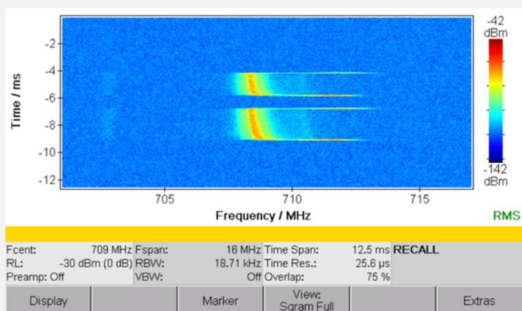
*Figure 2: Signal onset and dying down made clear by the High Resolution Spectrogram of the IDA2*
