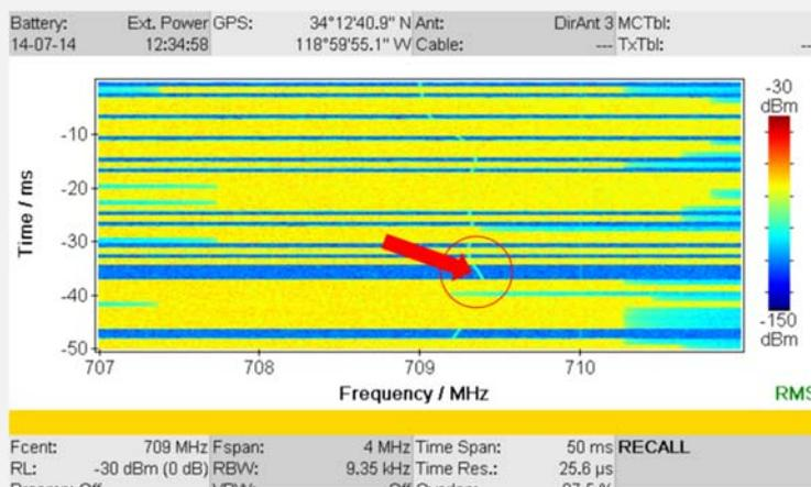
Figure 6: Signal clearly identifiable even with full LTE traffic
