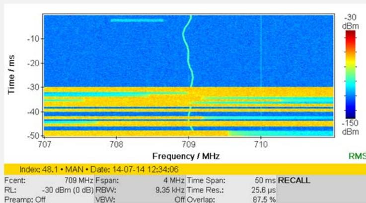
Figure 5: Time-continuous High Resolution Spectrogram uncovers the emissions from a bag sealer between the LTE payload signals
