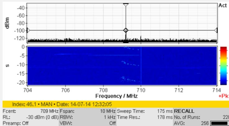
Figure 4: Frequency-agile interference signal between 708 MHz and 710 MHz
