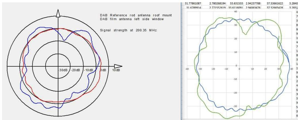
**Figure 1: The resulting circular plot in the measurement documentation provides the TE engineers with valuable information about how well an antenna receives a signal according to the angle of incidence in the real installation situation. It shows the antenna gain  $G$ , and the instantaneous value of the field strength measured at the antenna output in [dB $\mu$ V].**
