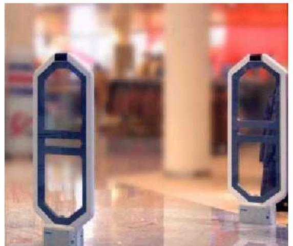
*Magneto acoustic gate used for product surveillance*
