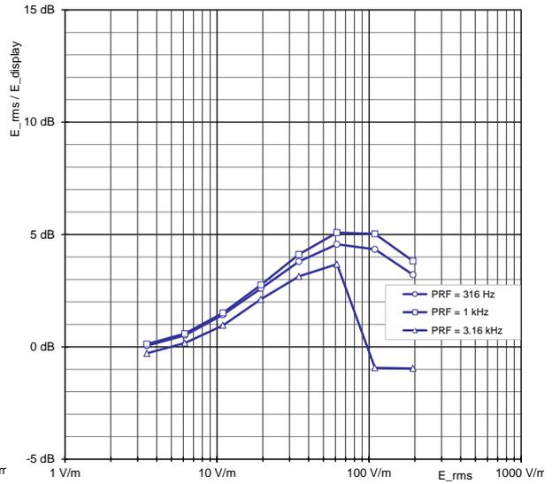
Display Deviation for Standing Radar Signals Duty Cycle 1 / 1000
