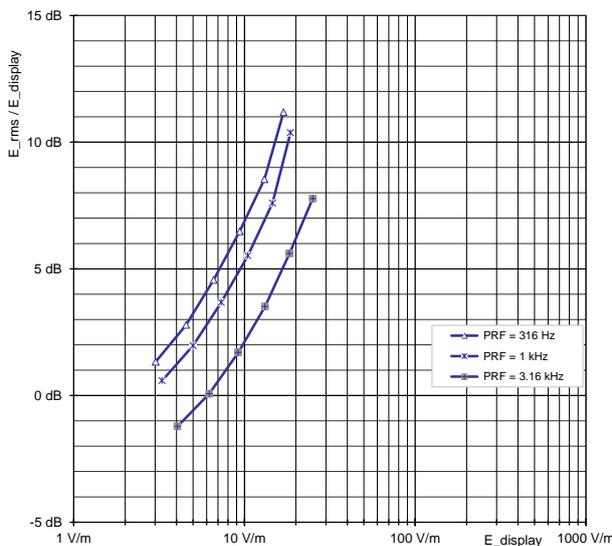
Display Deviation for Standing Radar Signals Duty Cycle 1 / 3162
